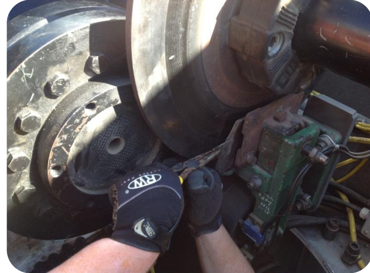
Brake Pad Replacement
